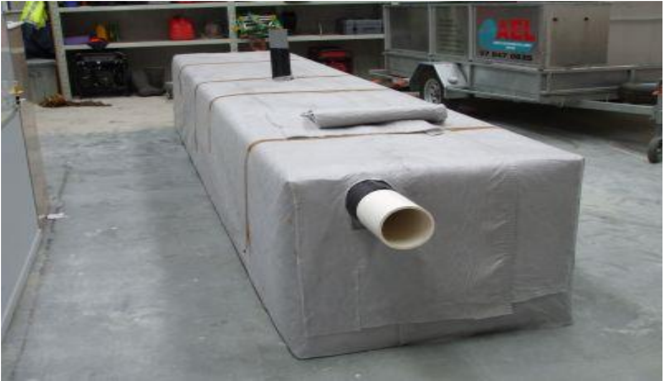
Modular tank assembly fabricated in the workshop, ready for installation.
